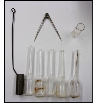
Testing bottles, beaker and caliper used with centrifuge.
